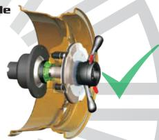
This is the correct handling. (example of application with QuickPlate)
