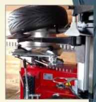
Mini roller can be used to gently drive stiff walled tires up and off the rim from the bottom
