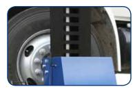
CLHM-135 & CLHM-185 Mechanical Lock Ladder 25 heavy-duty safety locks every 2-1/2" allow technicians to work at an ergonomic height to increase productivity and minimize fatigue.
