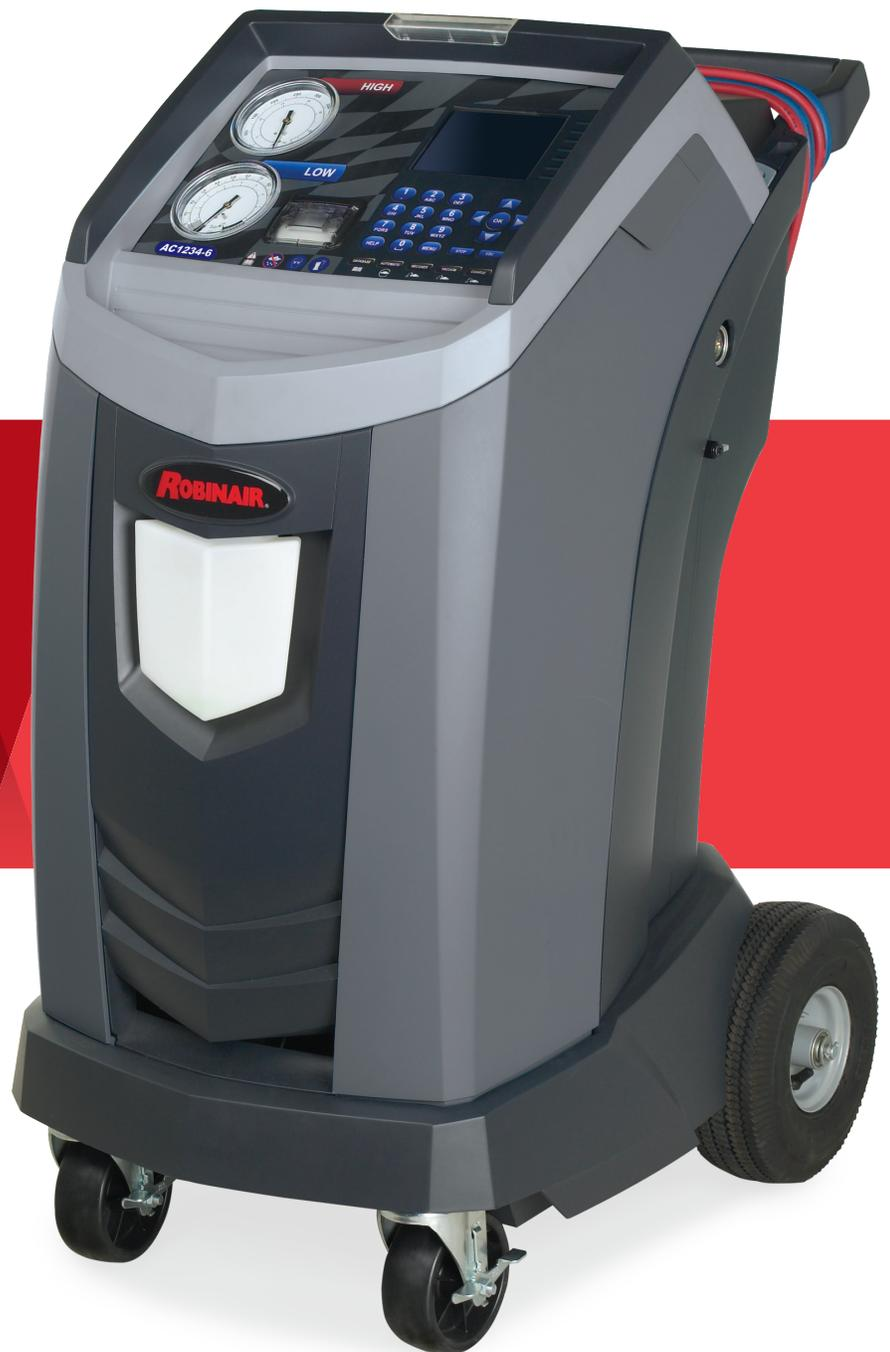
**Robinair recovery machines are the North American leaders in R-1234YF service.** The AC1234-6 and new AC1234-4 offer fully automatic operation, a powerful 1.5 CFM pump and use a liquid refrigerant flush function to recover more refrigerant faster. Both machines exceed J2843 requirements for R-1234YF recovery, recycle and recharge equipment. Standard features include an integrated refrigerant identifier, automatic internal tank refill, automatic oil drain and a color display.
